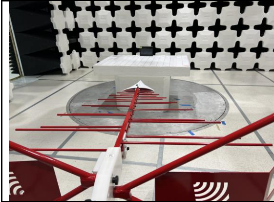
Radiated Emission Test below 1GHz Front View
