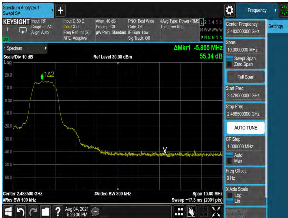
Plot 7-18. Band Edge Plot Antenna WF8 (Bluetooth with Hopping Disabled, 8DPSK, ePA – Ch. 78)
