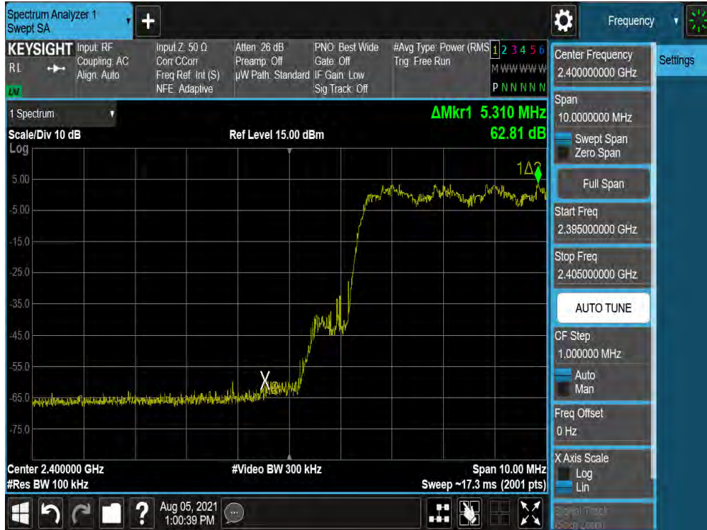
Plot 7-19. Band Edge Plot Antenna WF8 (Bluetooth with Hopping Enabled, 8DPSK, ePA)
