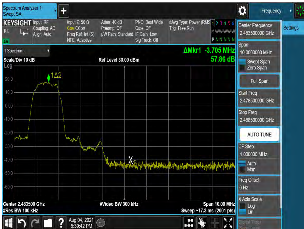
Plot 7-26. Band Edge Plot Antenna WF7 (Bluetooth with Hopping Disabled, 8DPSK, ePA – Ch. 78)
