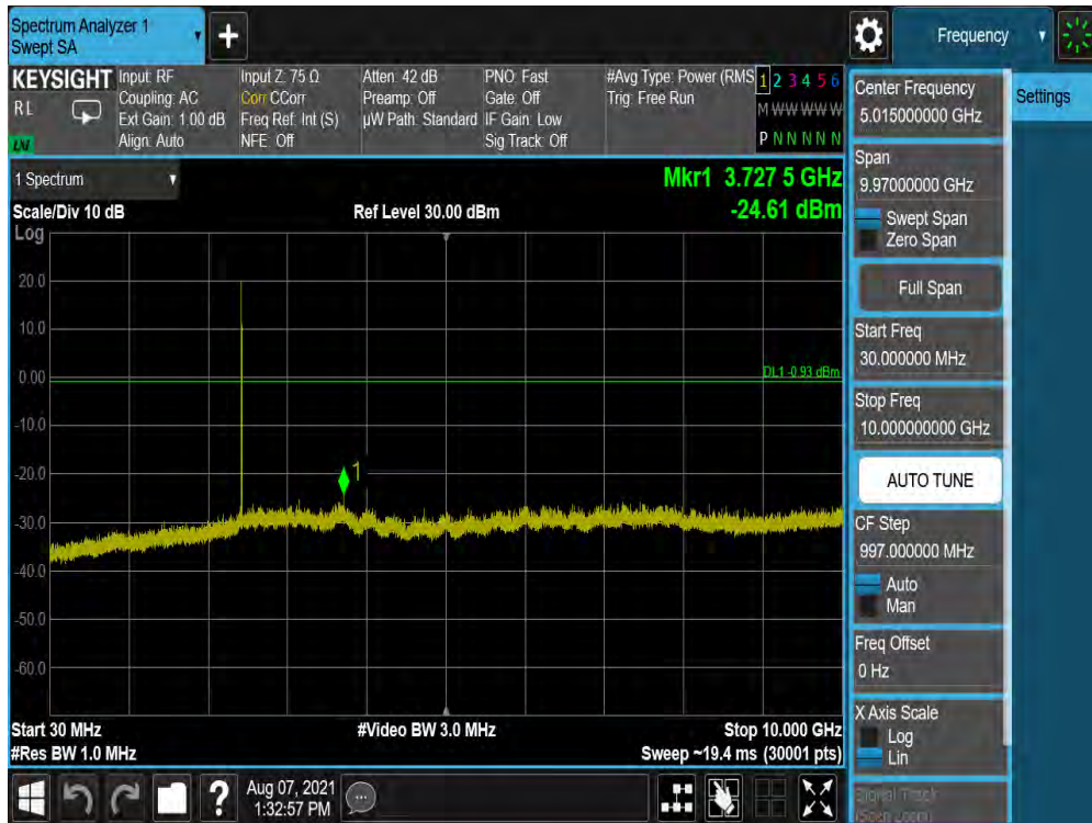
Plot 7-47. Conducted Spurious Plot Antenna WF8 (Bluetooth, GFSK, ePA – Ch. 39)
