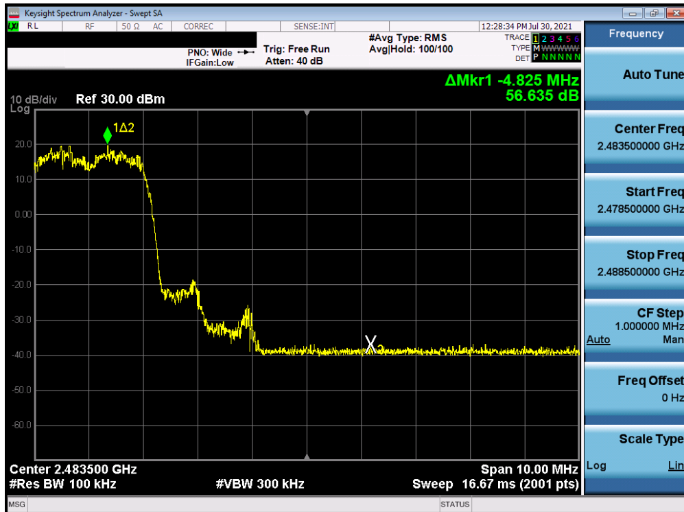
Plot 7-28. Band Edge Plot Antenna WF7 (Bluetooth with Hopping Enabled, 8DPSK, ePA)
