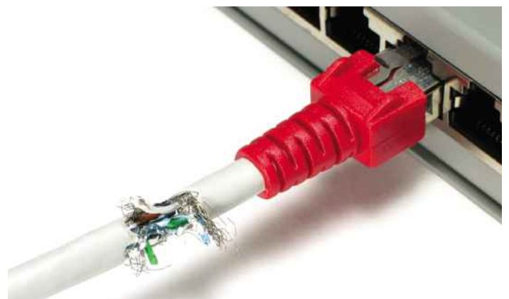
▲ Check your Ethernet cables for wear and tear
