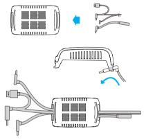
② Thread the separated strap through the HMD cable ports in turn and routed under the dedicated long connection cable, then the receiver end will be fixed on the HMD strap.
