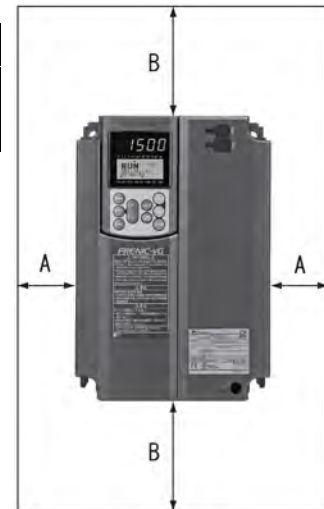
Figure 3.3-1 Mounting Direction and Required Clearances
