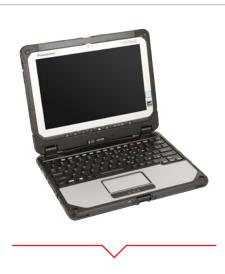
The RF-3577-76EN Rugged 10.1-inch Detatchable Laptop features a removable keyboard that transforms it into a tablet. This Windows® 10 device is equipped with an Intel® Core™ processor and includes Bluetooth® and wireless connectivity. The RF-3577-76EN meets MIL-STD-810G and is IP65 certified for water resistance.
