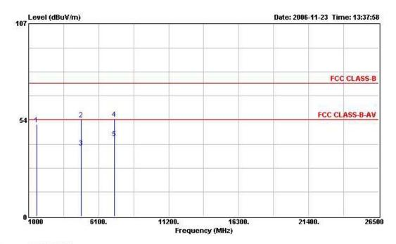
Condition : FCC CLASS-B 3m HORN-6903-04-09 VERTICAL
