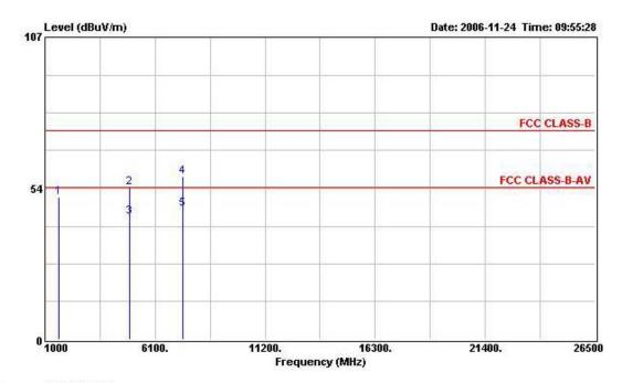
Condition : FCC CLASS-B 3m HORN-6903-04-09 VERTICAL
