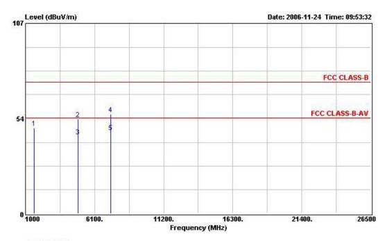
Condition : FCC CLASS-B 3m HORN-6903-04-09 VERTICAL
