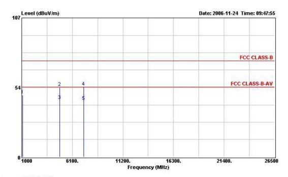
Condition : FCC CLASS-B 3m HORN-6903-04-09 VERTICAL
