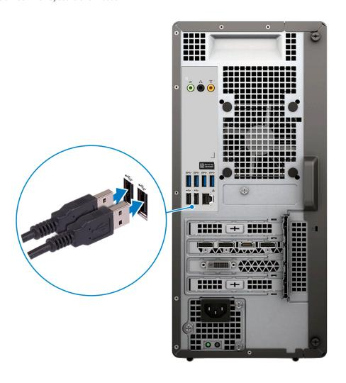
2. Connect to your network using a cable, or connect to a wireless network.
