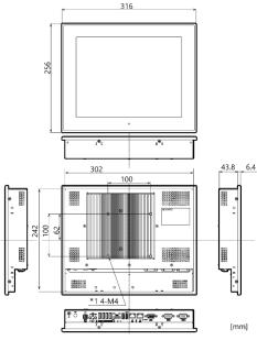
$^{\star 1}$  The maximum length that a screw can penetrate from the surface of the enclosure is 8 mm.
