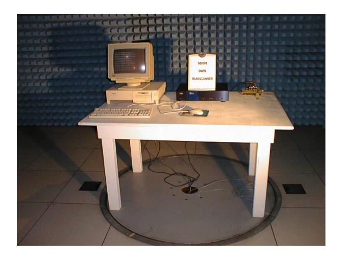
Radiated emission test (Front view)
