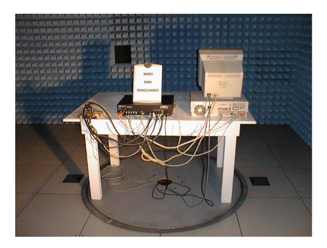
Radiated emission test (Rear view)
