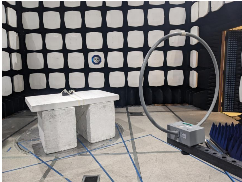
Figure1 – Test Set up - Radiated Emissions <30 MHz
