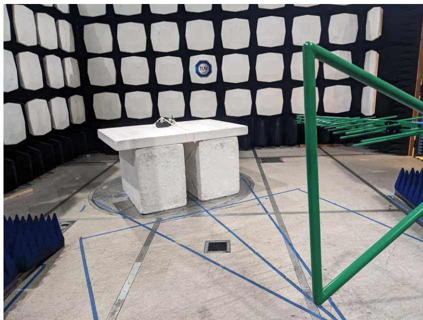
Figure2 – Test Set up - Radiated Emissions <1 GHz
