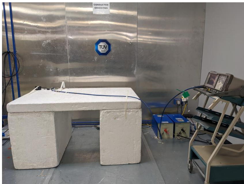
Figure 4 – Test Set up – Power Line Conducted Emissions
