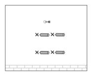
Insert the plastic wall anchors into the 6 mm diameter holes.
