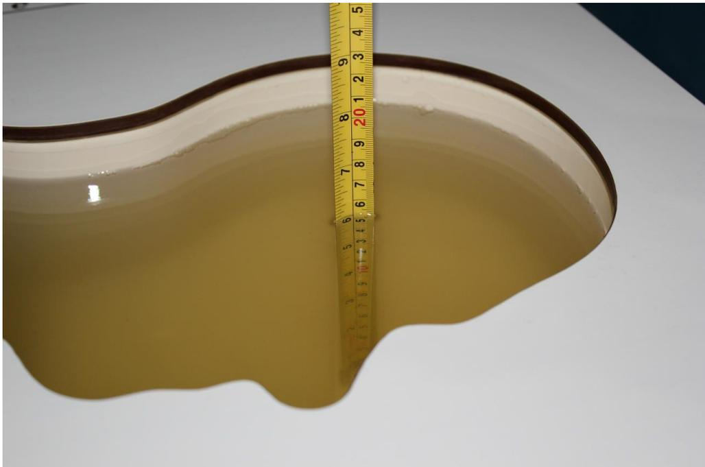
Picture 7-5: Liquid depth in the Head Phantom(2550MHz)
