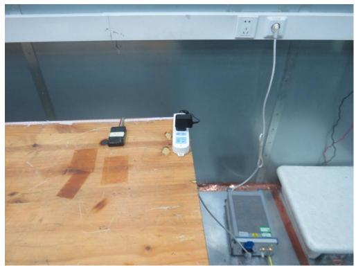
Picture 2: Conducted Emissions Test Setup
