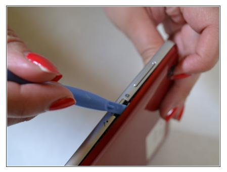
Remove the back cover by lifting with a plastic opening tool, below the camera button slot.
