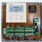
PCB, Power trans, Terminal block
