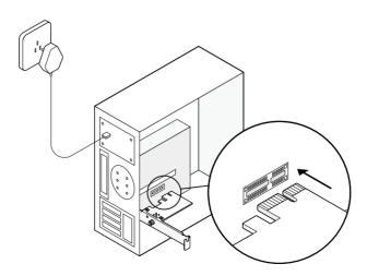
**4.** Locate an available **F\_USB** connector and carefully plug the USB cable into it.
