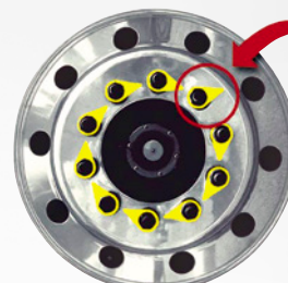
Loose and unsafe
