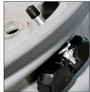
Valve options for 0.453", 0.625", and 7.7mm rim holes
