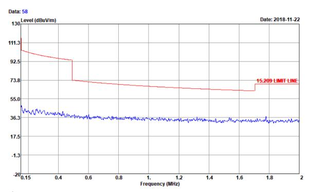
Condition : 15.209 LIMIT LINE 3m LOOP ANT\_1806 HORIZONTAL
