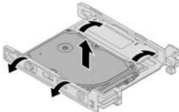
Figure 49. Removing the 2.5-inch storage drive from the bracket
