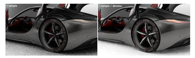
If you spend more samples per pixel rendering you will end up with less interactivity but also with less noise. The left image below is rendered at 16 spp and the denoiser applied to this image gives much better results as you see with the image on the right below.
