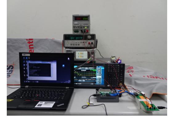
Conducted Setup Photo (Measurement at Antenna Port)\_2XS
