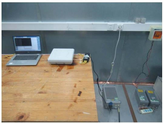
**Picture 2: Conducted Emissions Test Setup**
