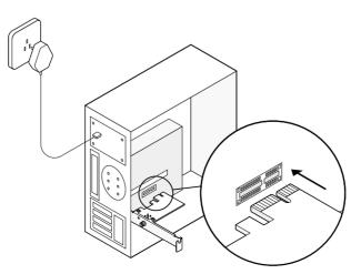
4. Locate an available F\_USB connector and carefully plug the Bluetooth USB cable into it.
