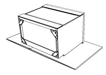
Install the four supplied feet via the four installation points. Make sure that each foot is securely fastened.
