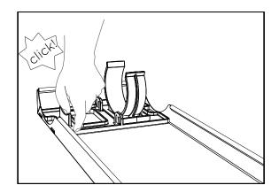
3 Make sure both clip modules are in the same orientation after installation.
