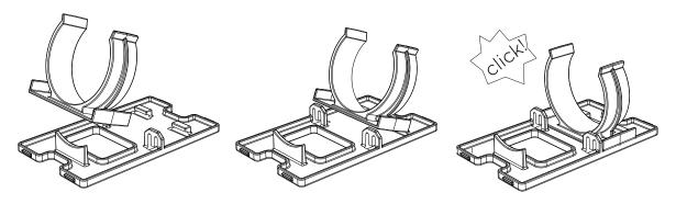
2 Press in both assembled clip modules into the kick panel in the orientation as shown below.
