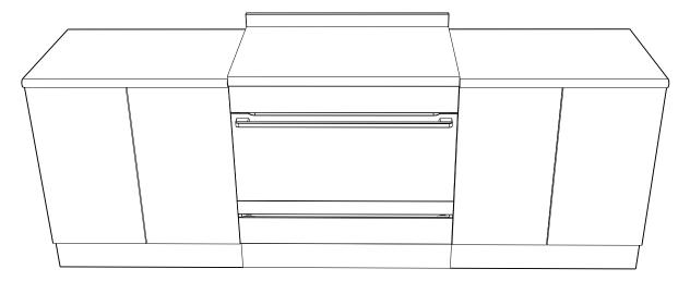
The slot-in type installation use the appliance as supplied. The appliance can be mounted on a plinth. This enables a continuous cupboard kickboard to be installed, giving a more intergrated appearance. There is no clearance requirement between oven and adjacent side cabinets.
