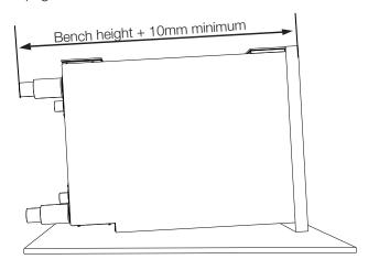
Tilt the appliance upright by lifting the back of the hob and pivoting it about the back two feet.
