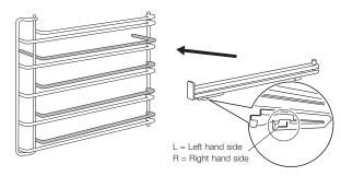
2 The shaded wires indicate the wire the slide can be mounted on. Fit slide rear clips to the rear of wire at an angle as shown below.
