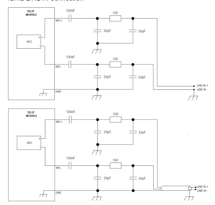
If the audio source is not a mike but a different device, the following connections can be done. Place 100nF capacitor in series with both inputs, so the DC current is blocked.
