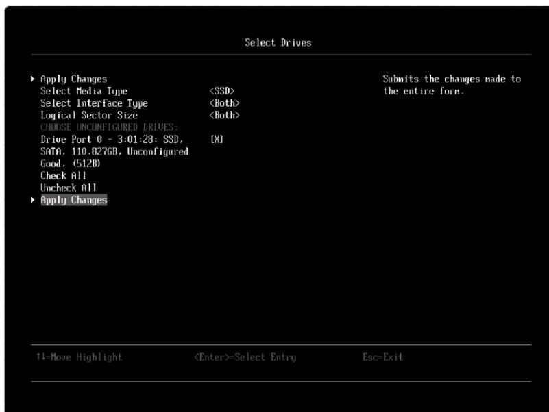
**Figure 20. Configuration of virtual drives**
