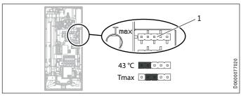
1 Jumper for anti-scalding protection setting
