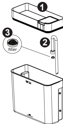
Disassembly water tank
