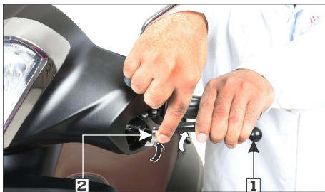
(1) Integrated brake lever (2) Lever lock
