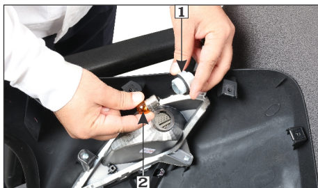
(1) Bulb holder (2) Front turn signal bulb
