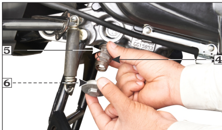
(4) Spring (5) Oil strainer screen (6) O-ring
