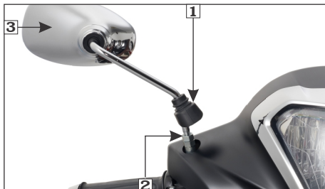
(1) Dust cover (2) Lock nut (3) Rear view mirror
