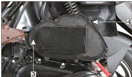
(3) Air cleaner element holder component (4) Air cleaner sub assembly case
