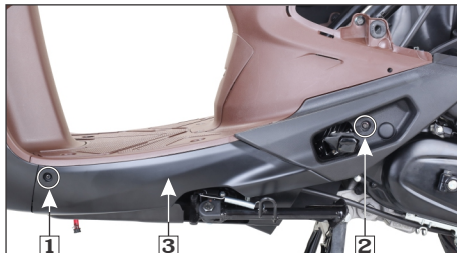
(1) Screw (2) Bolt (3) Floor side cover
