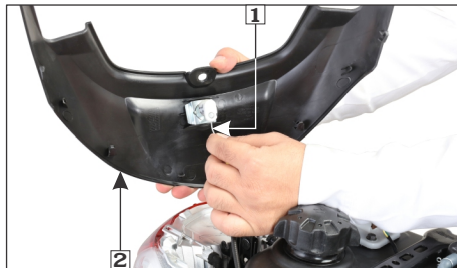
(1) Seat catch cable (2) Tail/stop lamp cover
