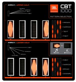
(Header position example shown above: Upper Half NARROW pattern setting; Lower Half DOWNFILL pattern setting; EQ is MUSIC/FLAT setting.)
