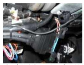
3. Connect the vehicle OBDII connector to the mating Solera OBDII connector
