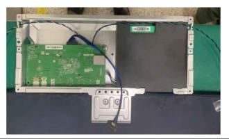
Assemble navi key and FFC LED to the PCBA key BD as the picture 1
