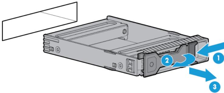
To replace the component, slide the component into the bay until it clicks.
