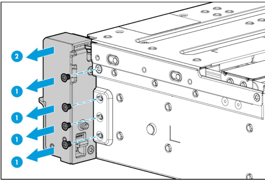
5. Remove the pull tab cage.
