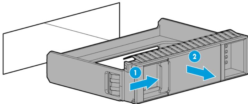
To replace the LFF drive blank, slide the component into the bay until it clicks.
