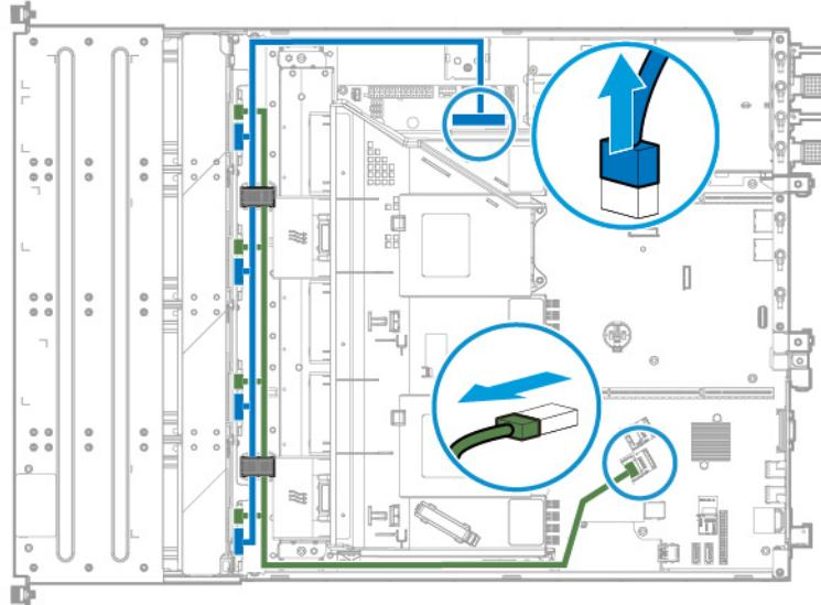
— 8-bay LFF non-hot-plug drive cable disconnections
