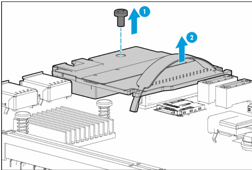
To replace the component, reverse the removal procedure. After installing the new dedicated iLO management module, enable the dedicated iLO connector ("Enabling the dedicated iLO management module" on page [65](#)).
