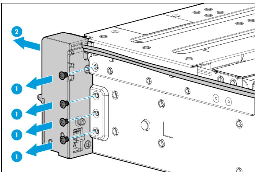
9. Remove the left quick-release latch rack ear.
