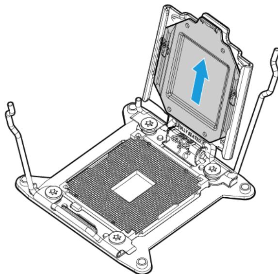
4. Install the processor. Verify that the processor is fully seated in the processor retaining bracket by visually inspecting the processor installation guides on either side of the processor. **THE PINS ON THE SYSTEM BOARD ARE VERY FRAGILE AND EASILY DAMAGED.**
