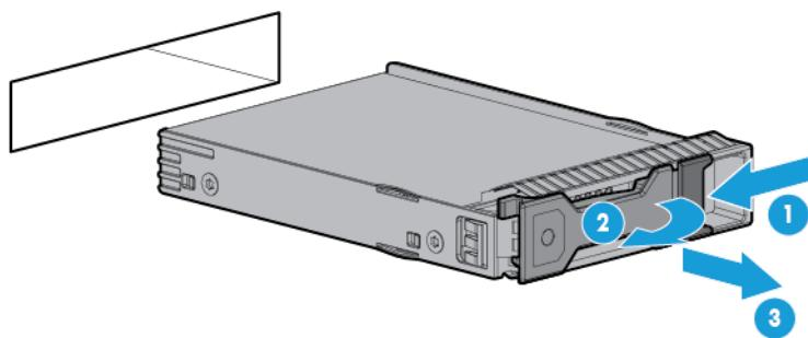
5. Remove the drive from the carrier.
