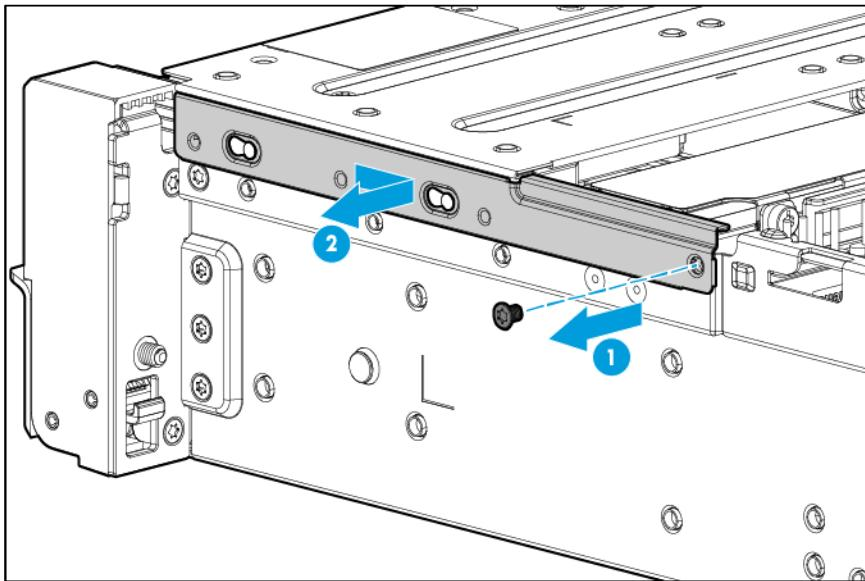
8. Remove the right quick-release latch rack ear assembly.
