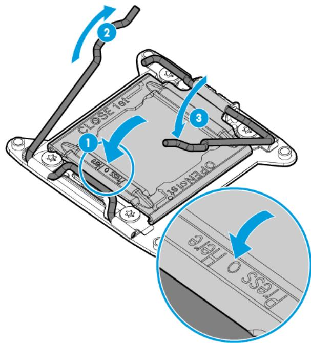
7. Install the processor socket cover onto the processor socket of the failed system board.
