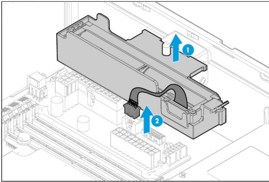
6. Remove the HP Smart Storage Battery from its holder.
