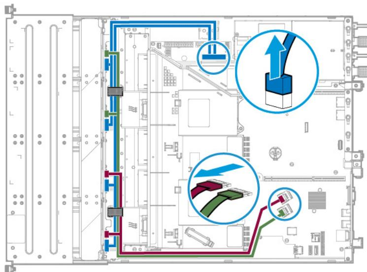
10. Remove the non-hot-plug drive cable assembly from the drive cage:
