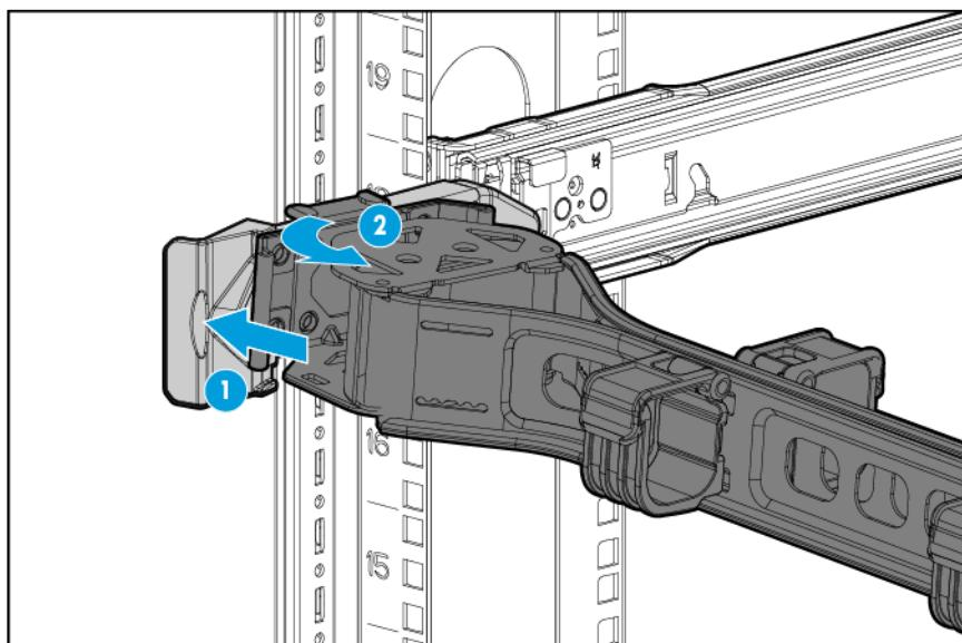
2. Open the cable management arm. The cable management arm can be right-mounted or left-mounted.
