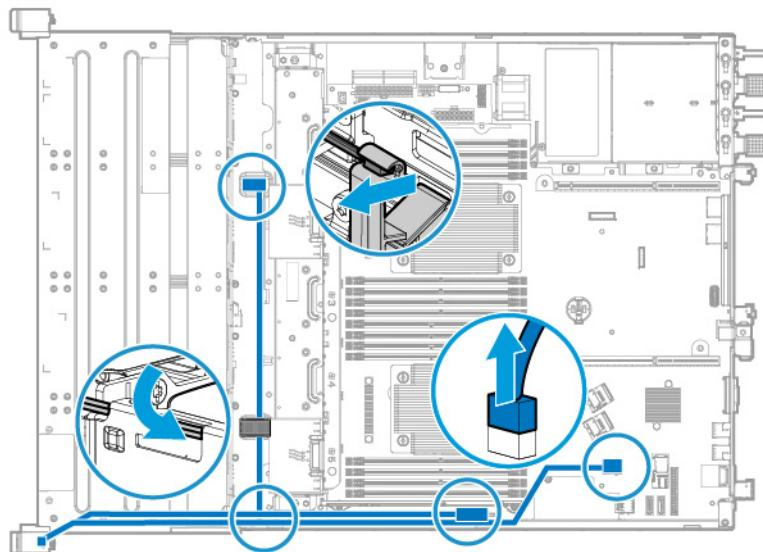
7. Remove the cable cover behind the right quick-release latch rack ear.
