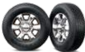
18-inch Polished Aluminum with Painted Pockets LEFT: Accent-Color Pockets Standard on Laramie Longhorn® with Two-Tone Exterior Paint (WBJ) RIGHT: Silver Pockets Standard on Laramie Longhorn with Available Monotone Exterior Paint (WBA)
