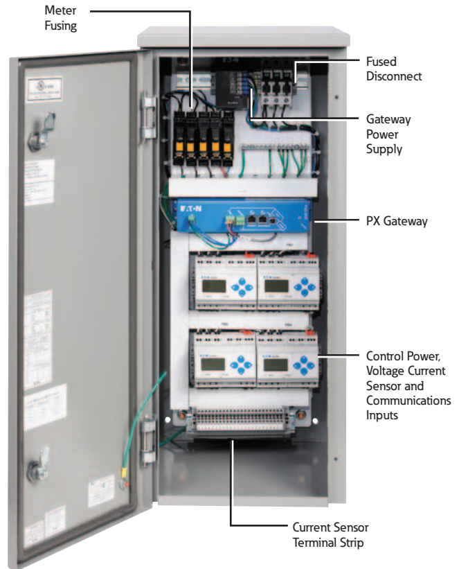
Multi-Unit Enclosed Meter, Inside View of IQ 35M
