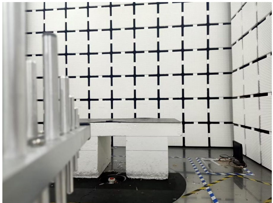
Radiation Emission Test Setup (30MHz to 1GHz)
