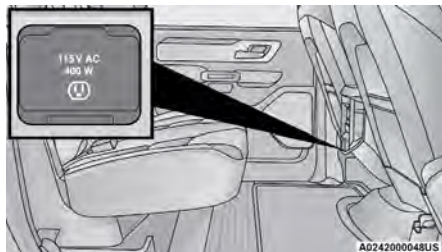
Rear Center Console Power Inverter Outlet (If Equipped)
