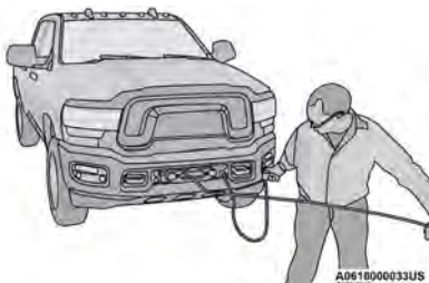
Pulling Synthetic Rope Under Tension
