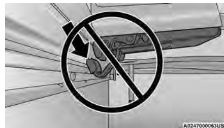
Improper Clamp Position
