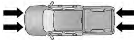
Jack / Extensions Placement
