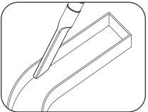
1 Before you begin, clean surfaces and remove all debris from the inside of the channel letter. Clean the surfaces with a 50:50 mixture of isopropyl alcohol (IPA) and water and let dry.
