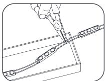
Measure and cut Select TX<sup>™</sup> LED strip to the appropriate length for each letter. Cuts can be made between any of the modules.
