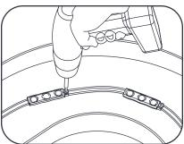
Use rivets, screws, or electrical grade RTV silicone to secure at least every third LED module within the channel letter. Use #6 (M3) or #4 pan headed metal screws, 1/8-inch (3.2 mm) rivets, or electrical grade RTV silicone.
