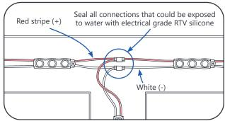
Connect LED strips using in-line (IDC) connectors or twist-on wire connectors.
