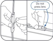
Remove tape backing and stick LED modules into place. When using tape apply approximately 15 psi pressure on the module (avoid the lens dome surface) for 5 seconds, full bonding strength after 24 hours. Continue until you have reached the end of the strip.
