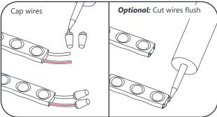
2 Must cap all exposed wires with appropriate wire connectors and seal with electrical grade RTV silicone.
