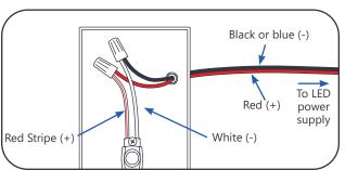
Connect the red stripe wire (+) of the LED strip to the red wire (+) of the power supply. Connect the white wire (-) of the LED strip to the black or blue wire (-) of the LED power supply.
