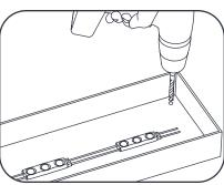
Drill a 1/4-inch (6.4 mm) hole near the LED strip and grommet the hole for supply wire access.
