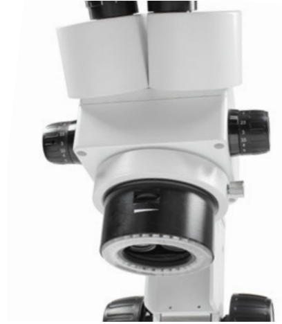
Dimmable, integrated LED ring illumination
