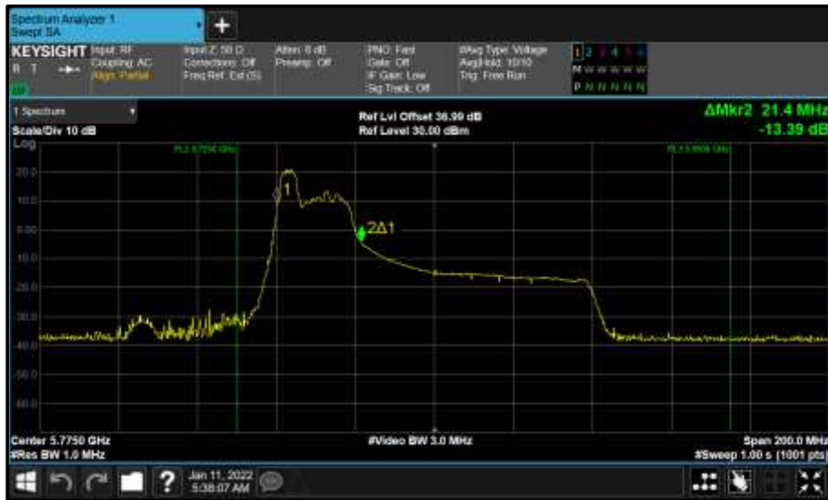
Figure 868 - Core 0 (A) 5775 MHz (CH155) 99% Bandwidth
