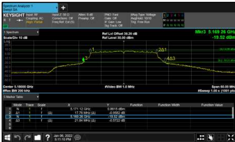
Figure 893 - Core 1 (B) 5180 MHz (CH36) 26 dB and 99% Bandwidth
