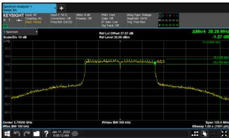
Figure 761 - Core 0 (A) 5795 MHz (CH159) 6 dB Bandwidth
