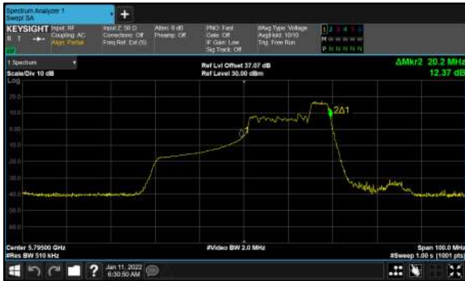
Figure 820 - Core 0 (A) 5795 MHz (CH159) 99% Bandwidth
