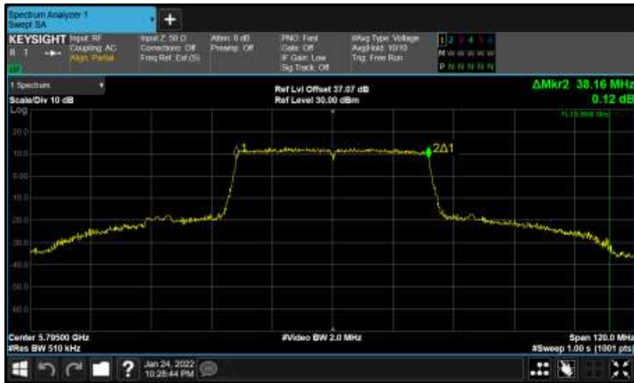
Figure 782 - Core 0 (A) 5795 MHz (CH159) 99% Bandwidth
