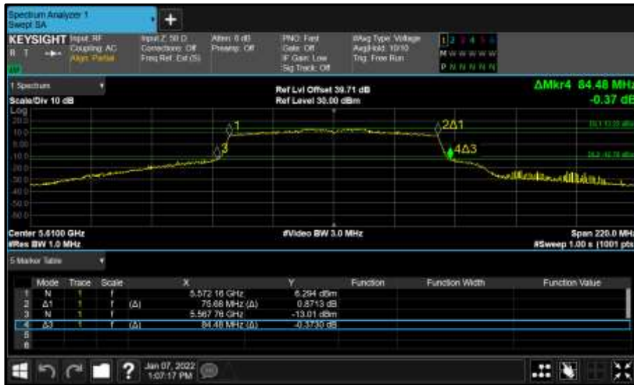
Figure 940 - Core 0 (A) 5610 MHz (CH122) 26 dB and 99% Bandwidth
