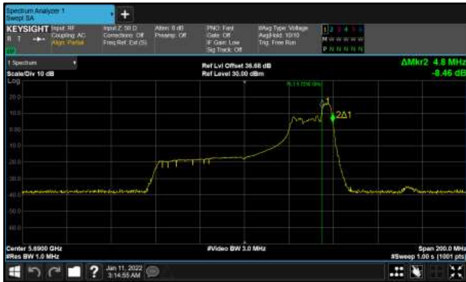
Figure 870 - Core 0 (A) 5690 MHz (CH138) 99% Bandwidth
