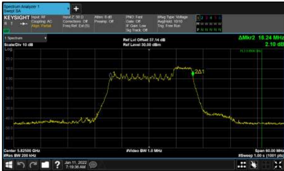
Figure 754 - Core 1 (B) 5825 MHz (CH165) 99% Bandwidth
