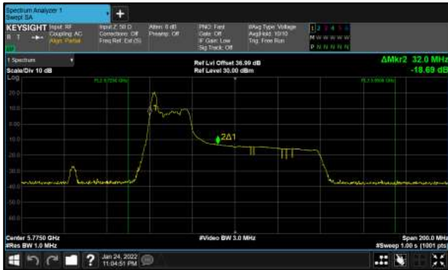
Figure 862 - Core 0 (A) 5775 MHz (CH155) 99% Bandwidth
