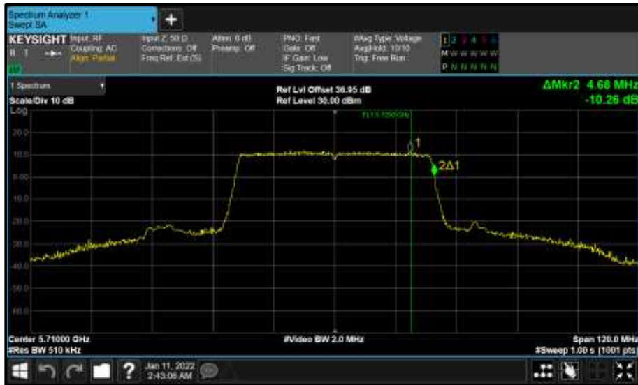
Figure 764 - Core 1 (B) 5710 MHz (CH142) 99% Bandwidth
