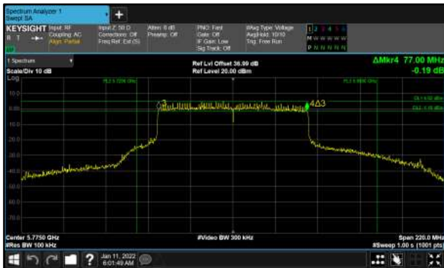
Figure 845 - Core 0 (A) 5775 MHz (CH155) 6 dB Bandwidth
