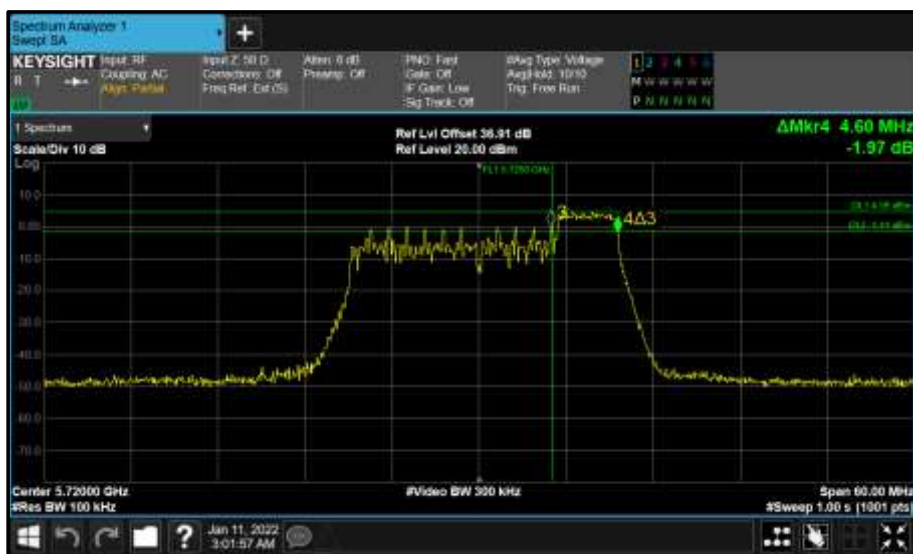
Figure 727 - Core 1 (B) 5720 MHz (CH144) 6 dB Bandwidth
