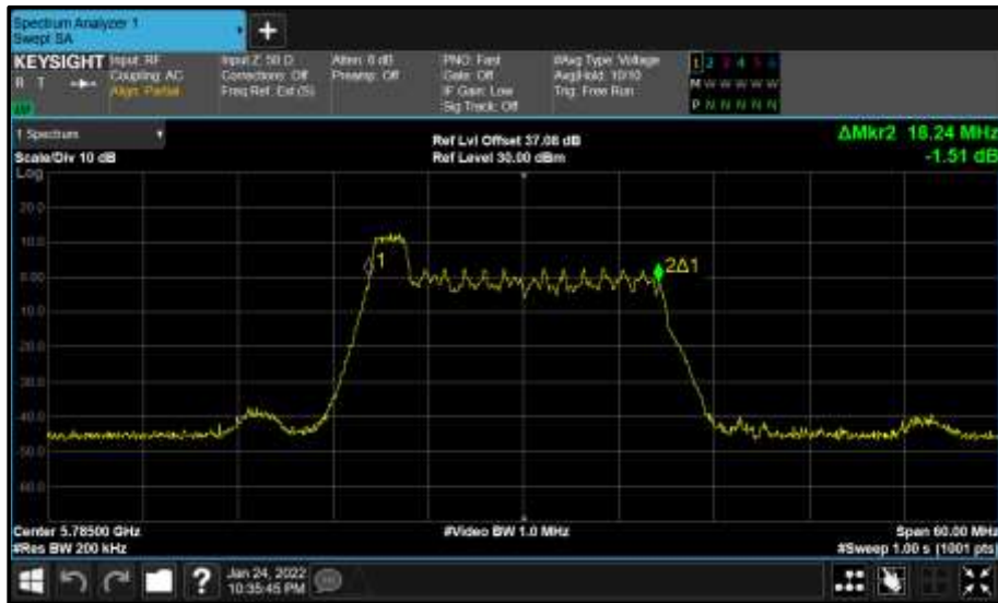
Figure 710 - Core 1 (B) 5785 MHz (CH157) 99% Bandwidth
