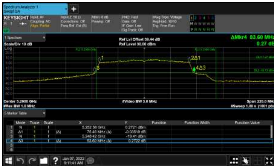
Figure 921 - Core 1 (B) 5290 MHz (CH58) 26 dB and 99% Bandwidth
