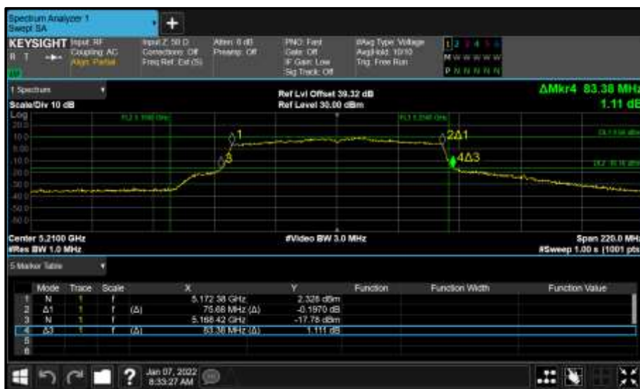
Figure 907 - Core 1 (B) 5210 MHz (CH42) 26 dB and 99% Bandwidth
