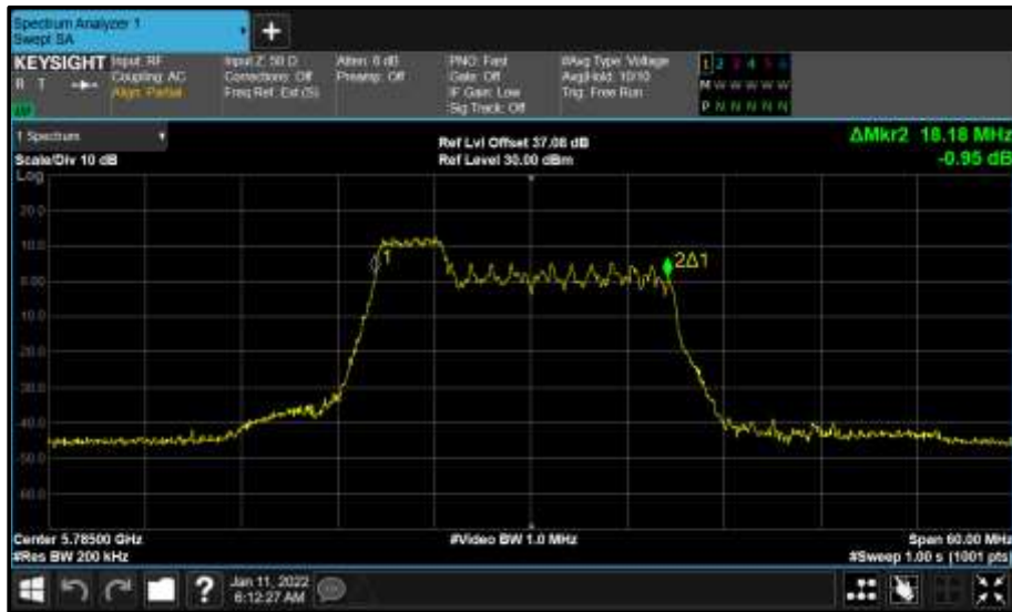
Figure 734 - Core 1 (B) 5785 MHz (CH157) 99% Bandwidth
