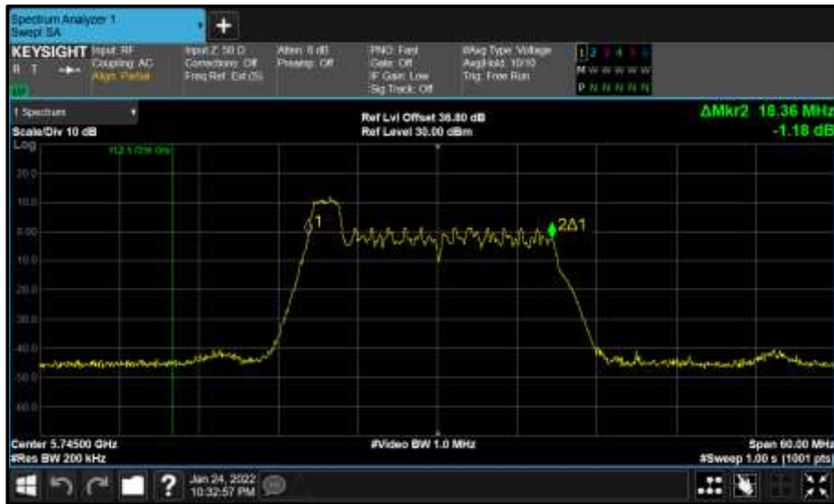
Figure 704 - Core 0 (A) 5745 MHz (CH149) 99% Bandwidth
