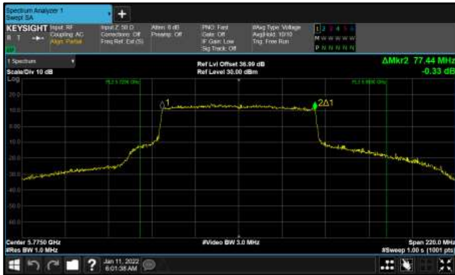
Figure 844 - Core 0 (A) 5775 MHz (CH155) 99% Bandwidth
