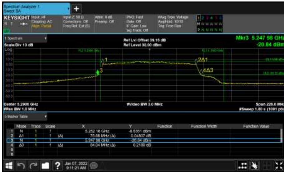
Figure 920 - Core 0 (A) 5290 MHz (CH58) 26 dB and 99% Bandwidth
