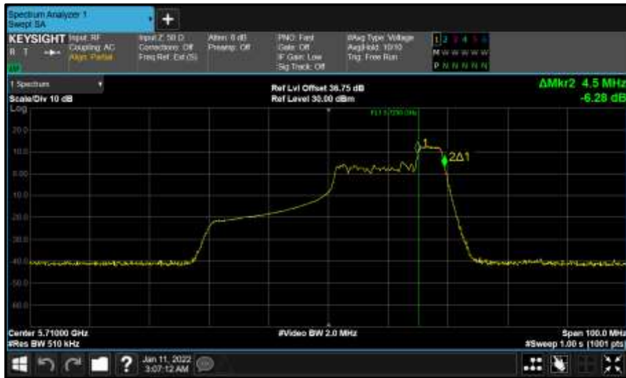
Figure 812 - Core 0 (A) 5710 MHz (CH142) 99% Bandwidth
