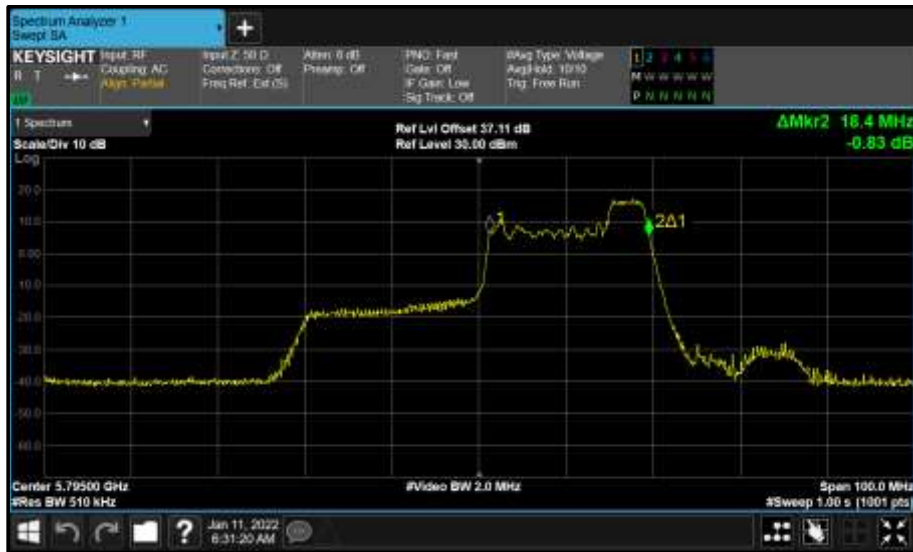
Figure 822 - Core 1 (B) 5795 MHz (CH159) 99% Bandwidth
