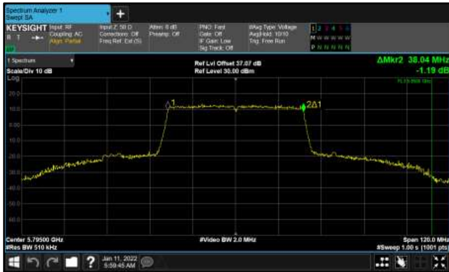
Figure 770 - Core 0 (A) 5795 MHz (CH159) 99% Bandwidth
