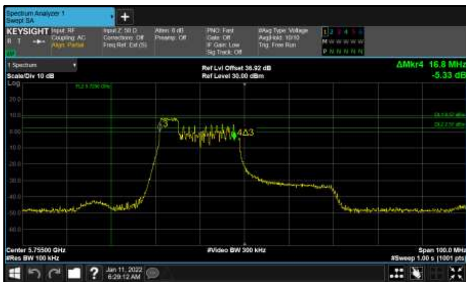
Figure 819 - Core 1 (B) 5755 MHz (CH151) 6 dB Bandwidth
