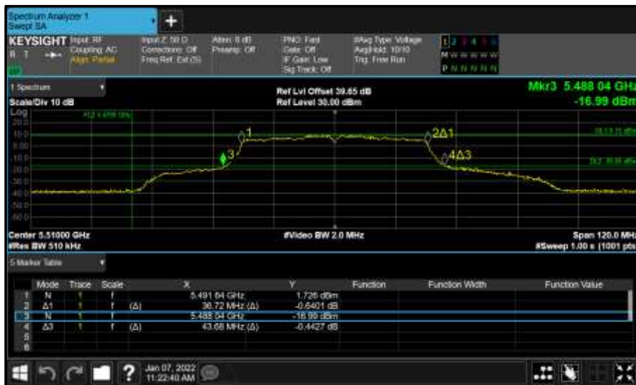
Figure 931 - Core 1 (B) 5510 MHz (CH102) 26 dB and 99% Bandwidth
