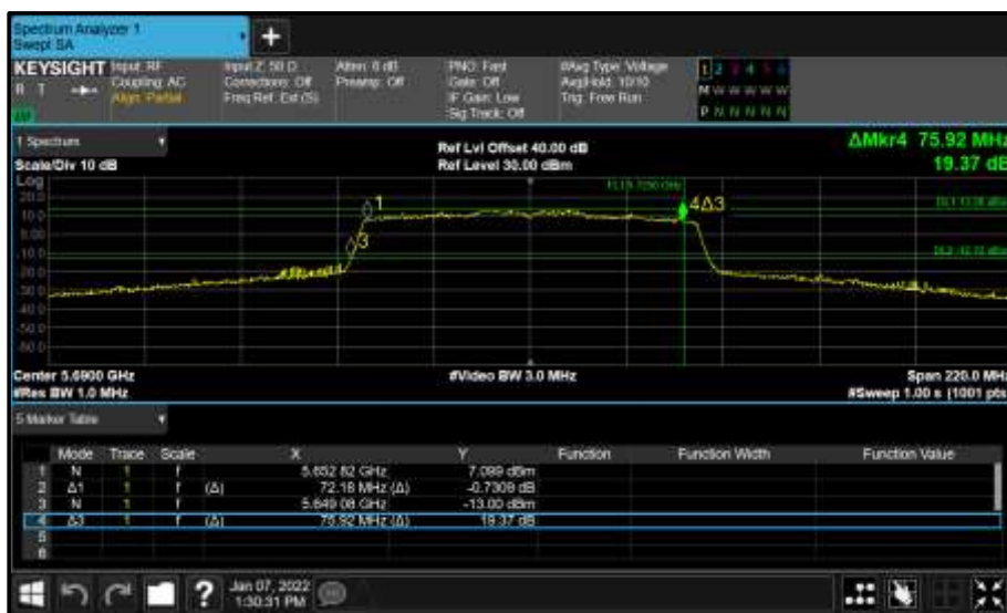
Figure 943 - Core 1 (B) 5690 MHz (CH138) 26 dB and 99% Bandwidth
