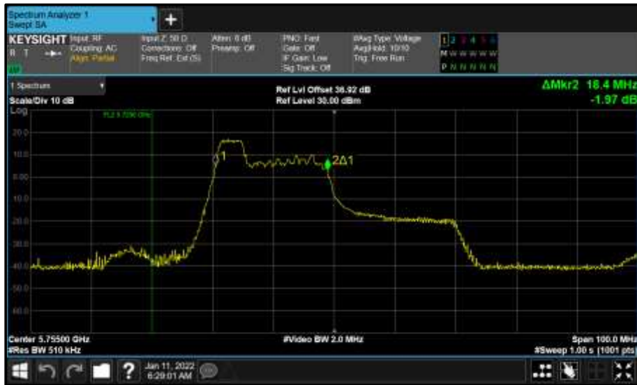
Figure 818 - Core 1 (B) 5755 MHz (CH151) 99% Bandwidth
