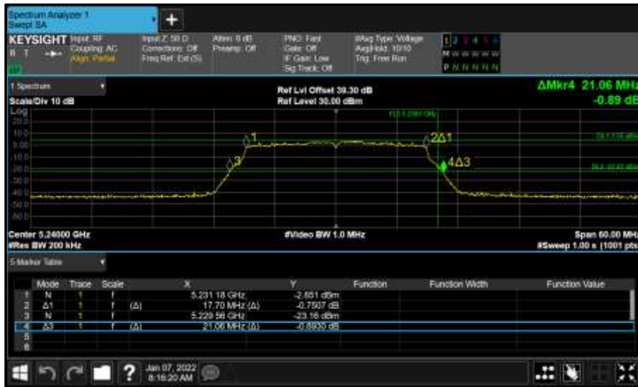
Figure 890 - Core 0 (A) 5240 MHz (CH48) 26 dB and 99% Bandwidth
