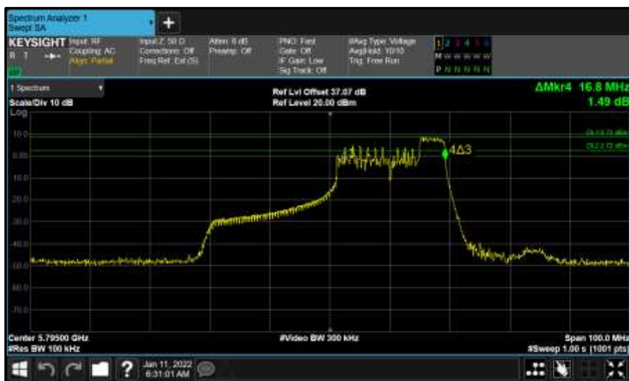
Figure 821 - Core 0 (A) 5795 MHz (CH159) 6 dB Bandwidth
