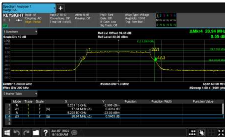
Figure 891 - Core 1 (B) 5240 MHz (CH48) 26 dB and 99% Bandwidth
