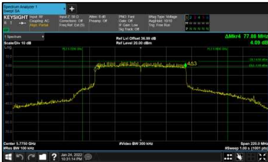
Figure 853 - Core 0 (A) 5775 MHz (CH155) 6 dB Bandwidth
