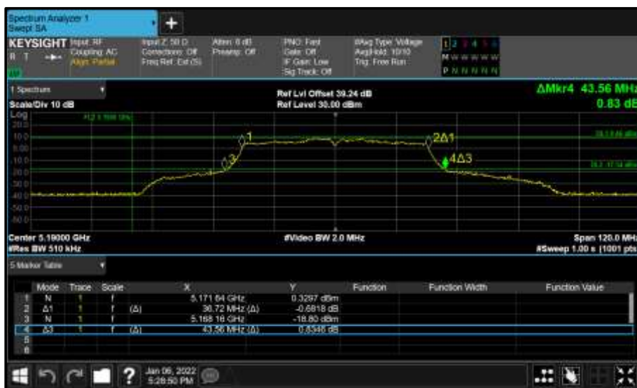
Figure 903 - Core 1 (B) 5190 MHz (CH38) 26 dB and 99% Bandwidth
