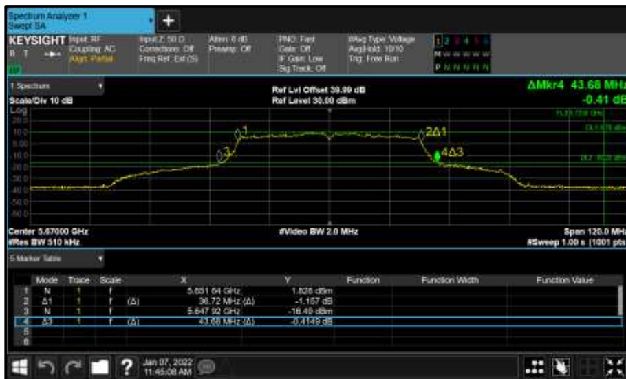
Figure 935 - Core 1 (B) 5670 MHz (CH134) 26 dB and 99% Bandwidth
