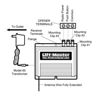
NOTE: With the transformer, use a 2 wire connection ONLY. Attach mounting clips to the receiver terminals 1 and 2, and to the opener terminals used for push button controls. Plug the transformer into the receiver as shown, and into a 120 Volt outlet.
