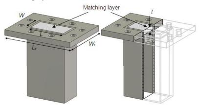
Figure 1: Validation Waveguide Dimensions
