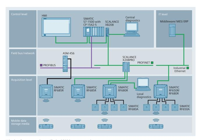
Whether for automation or IT, the RF600 system can be seamlessly integrated into your existing environment.
