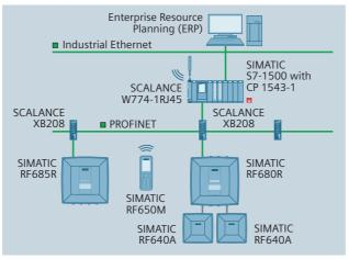
Exemplary configuration for an assembly line with SIMATIC RF600, SCALANCE W and SCALANCE X
