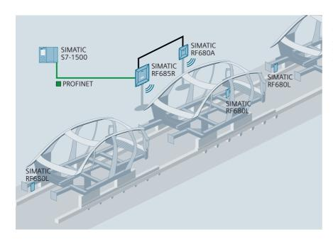
Consistent, end-to-end identification of car bodies, from the shell construction to the final assembly
