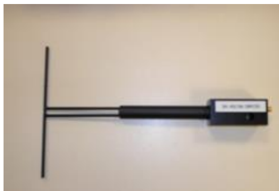
Figure 1 – MVG COMOSAR Validation Dipole
