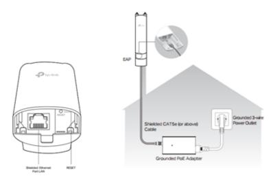
So for the latest hardware version, we suggest you use shielded CAT5e (you need to buy it yourself) and three phase supply (with grounding wire) for grounding. The grounding cable is not suitable for the latest hardware version since the grounding terminal has been deleted.
