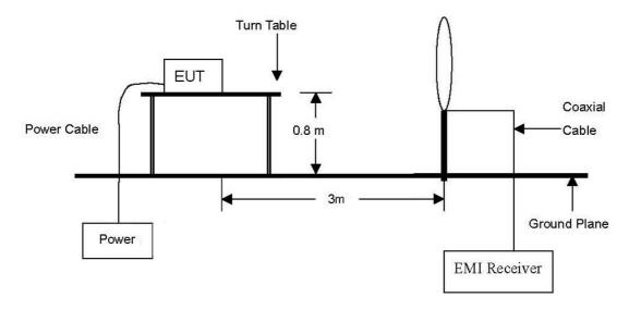
The diagram below shows the test setup that is utilized to make the measurements for emission from 30  $\,\text{Mb}$  to 1  $\,\text{GHz}$  Emissions.
