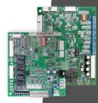
7. Aurora Controls: The powerful Aurora Base Control (ABC) offers two way communication between components, advanced operating logic and robust troubleshooting capabilities. The Aurora Expansion Board (AXB) adds support for true energy monitoring as well as compatibility with the Symphony Home Comfort Platform and our IntelliZone2 zoning system.
