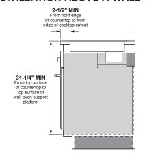
to nameplate for MIN. clearance to rear wall.
