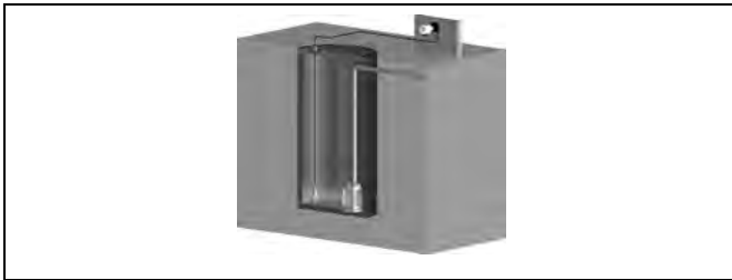
Fig. 5: Level measurement in a pump shaft with VEGAWELL 72, remote indication and adjustment with VEGADIS 12
